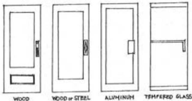
Appropriate Replacement Doors
