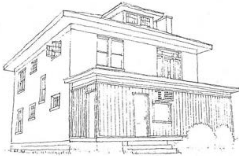
Inappropriate Porch Enclosure
